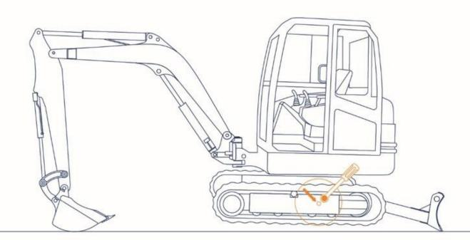
You will find a grease nipple at the side of the frame which is often covered by a cap. To remove the track's tension you have to untighten the nipple until grease leaks.
