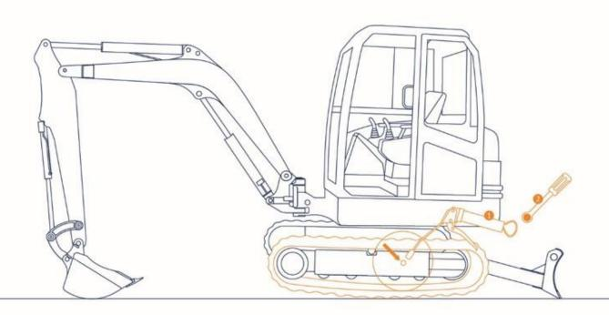
At last tighten the track. Therefore, fill the tension cylinder using a grease piston.
