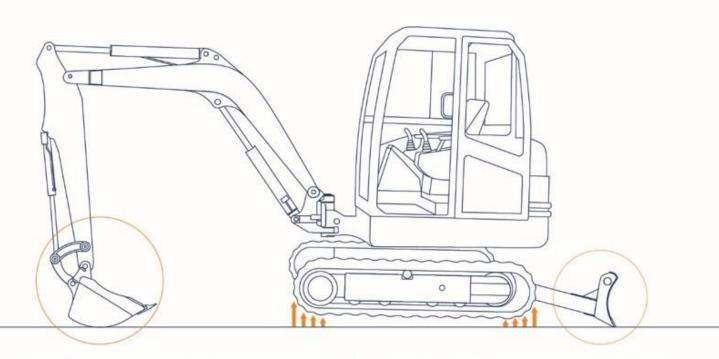
Firstly jack up your machine. Use boom and shield to lift the excavator until it loses ground contact.
