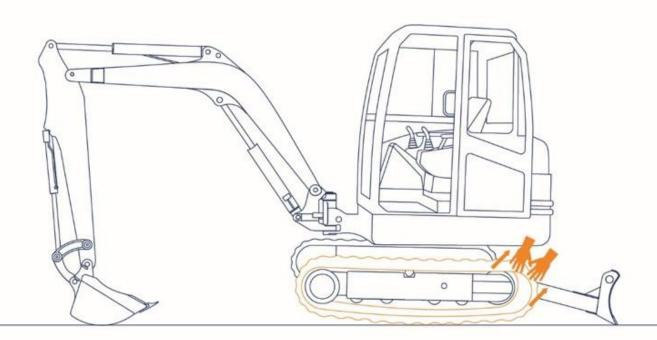
Now you can mount the new track. Mount the track from the sprocket in the direction of the idler.
